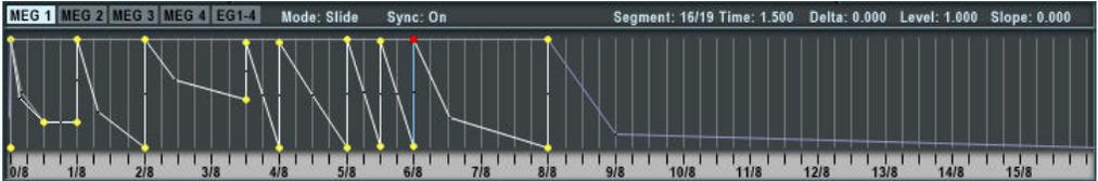
TERA provides you with four multi segment envelopes which can be used as a modulation source for many purposes. The envelopes can have up to 64 time/level segments giving you all from simple Attack/Decay style envelopes up to complex rhythmical patterns which can even be synchronized to MIDI tempo.
