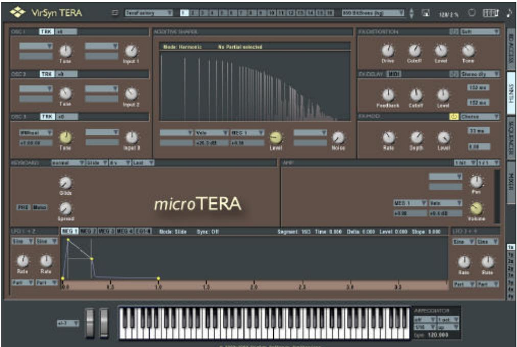
The waveshaper is the core of microTERA's synthesis engine. It works as a distortion unit that takes (for example) a sine wave as input and delivers an arbitrary spectrum as output. In contrast to other synths using also the waveshaping synthesis, microTERA uses a new technique to define the output spectrum of the waveshaper.
