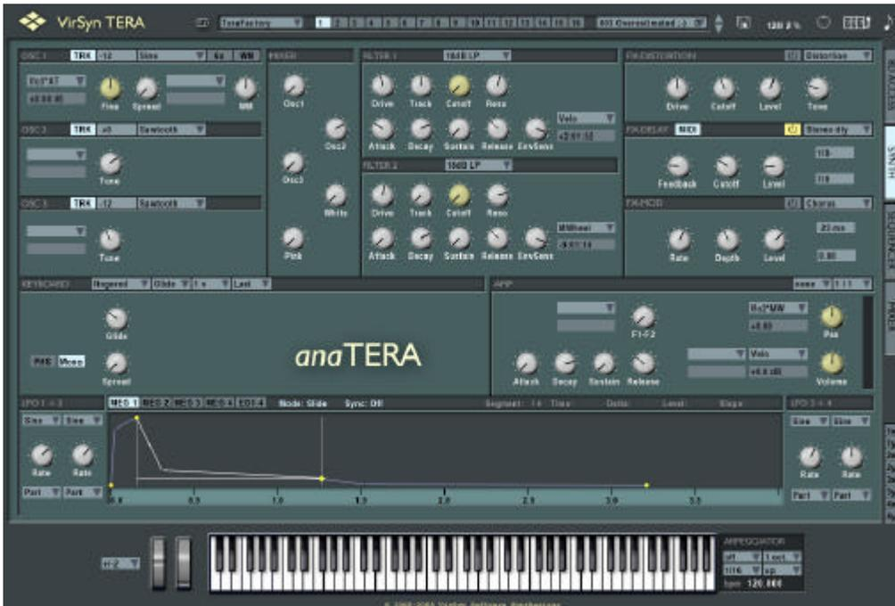
This synth is an enhanced classically modelled analogue synth. The 3 main oscillators of TERA are feeding the 2 standard multimode filters in parallel. The output of both filter modules can then be morphed for the resulting output. But keep in mind that despite this simple base structure you can do much more than with any previously existing analogue synths due to the multi-segment envelopes and the possibility to specify your own waveforms for each oscillator.
